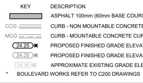
ASPHALT 100mm (60mm BASE COURSE & 40mm TOP LIFT) CURB - NON MOUNTABLE CONCRETE CURB & GUTTER \* CURB - MOUNTABLE CONCRETE CURB & GUTTER \* PROPOSED FINISHED GRADE ELEVATION - MOTI PROPOSED FINISHED GRADE ELEVATION - BOULEVARD \* APPROXIMATE EXISTING GRADE ELEVATION
